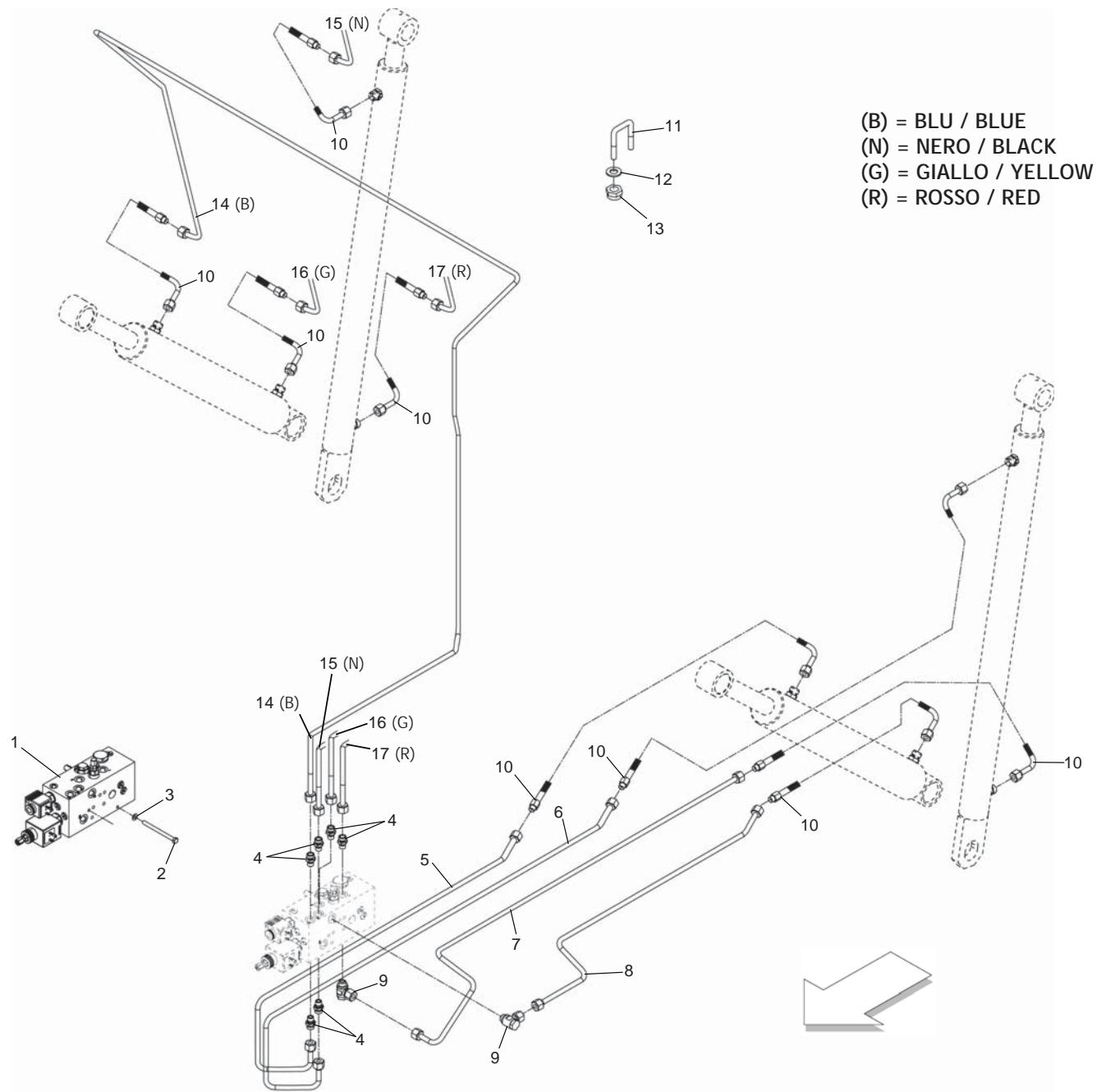
**IMPIANTO IDRAULICO MACCHINA (PARTE 1)**
