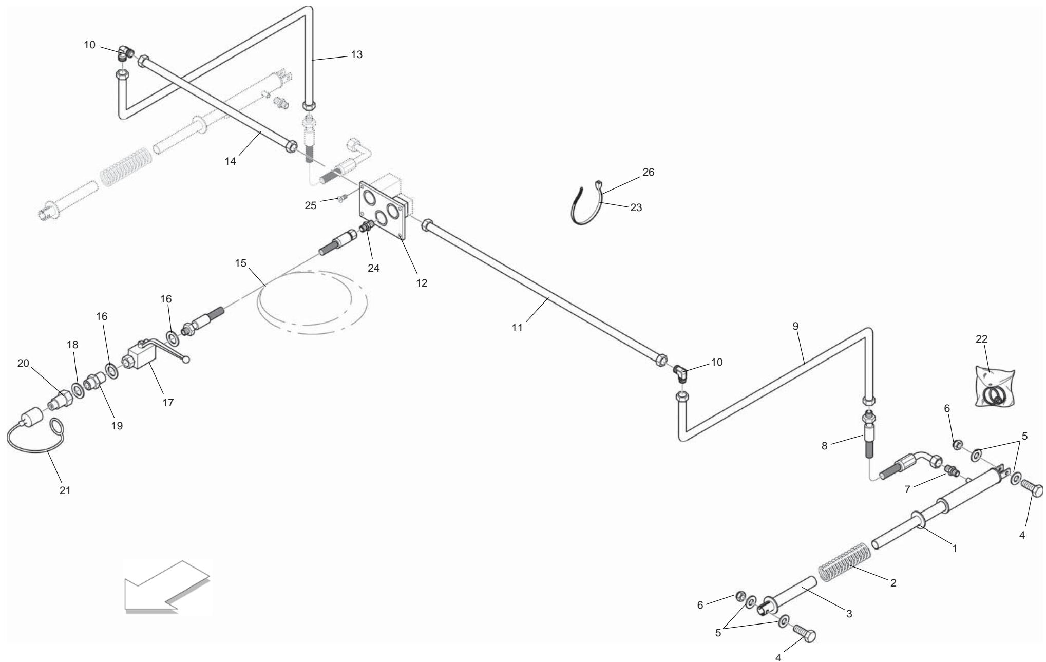
**IMPIANTO IDRAULICO PICK-UP**
