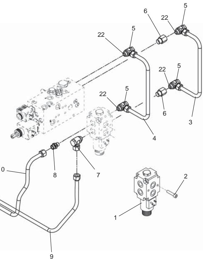
**IMPIANTO IDRAULICO MACCHINA (PARTE 2)**
