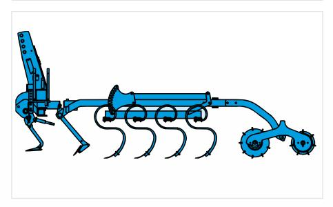
The System Korund seed bed combination with its versatile equipment options and range of working widths, is a powerful alternative in the area of soil preparation. Parallel linkage of the implement sections provides good contour following and uniform working
