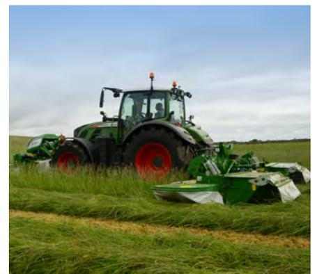
The Pro Glide range of rear mowers are fitted with patented ground adaption technology, which allows the bed to move back and up if the bed encounters small obstacles. This saves time and maximises throughput as it means the obstacle does not trigger the main break back protection. This results in higher mowing speeds being able to be achieved without the interruption of having to reset the break back.
