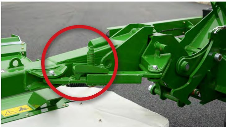
The Pro Glide rear suspension springs react instantly to ground contours, which results in a high quality cut even when working at high ground speeds. This allows the mowers to easily mow on rough or undulating terrain and still deliver optimum results.
