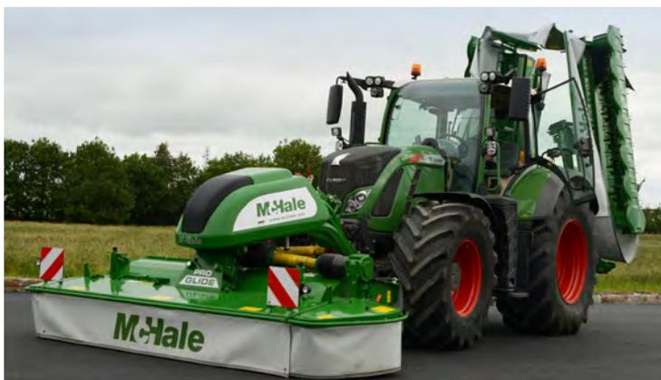
For transportation, the McHale Pro Glide folds vertically to position itself behind the centre point of the tractor for safe transport.
